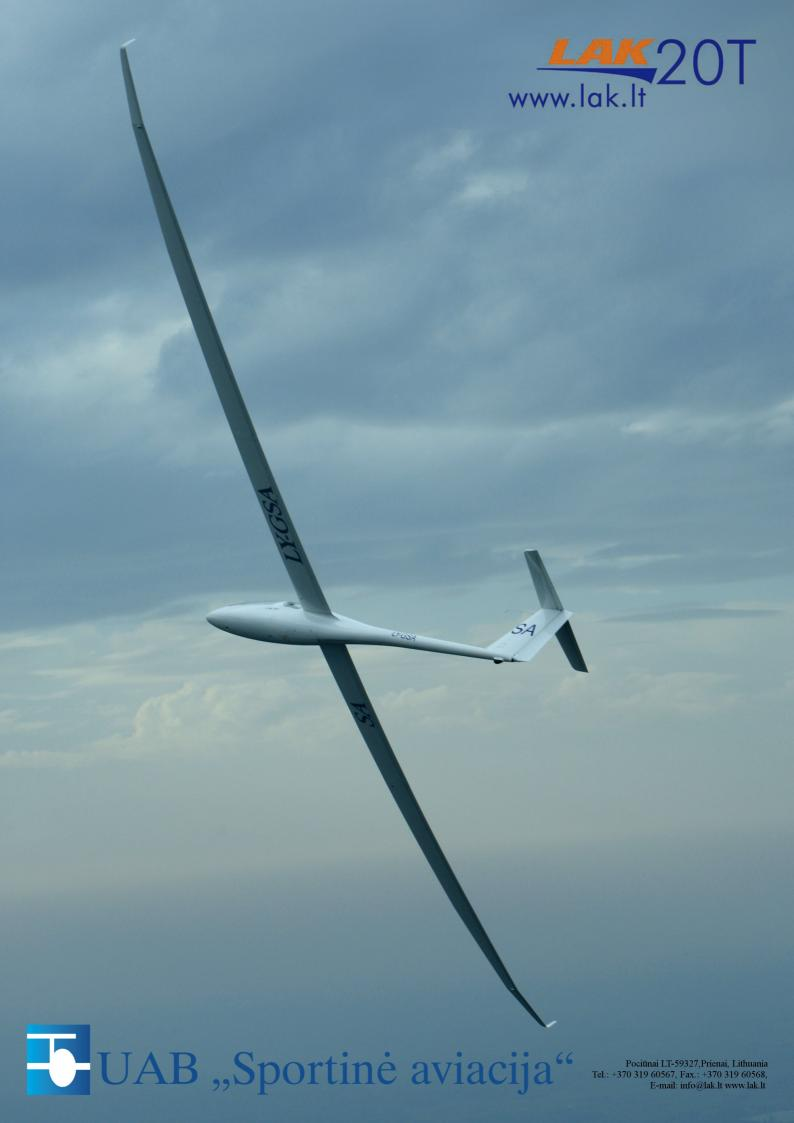
The LAK-20T is the newest JSC "Sportine aviacija" sailplane. The open class two-seat LAK-20 is designed to meet the latest standards of the gliding industry. The sailplane has a normal aerodynamic configuration with a "T" tail, and with wings slightly swept forward.
